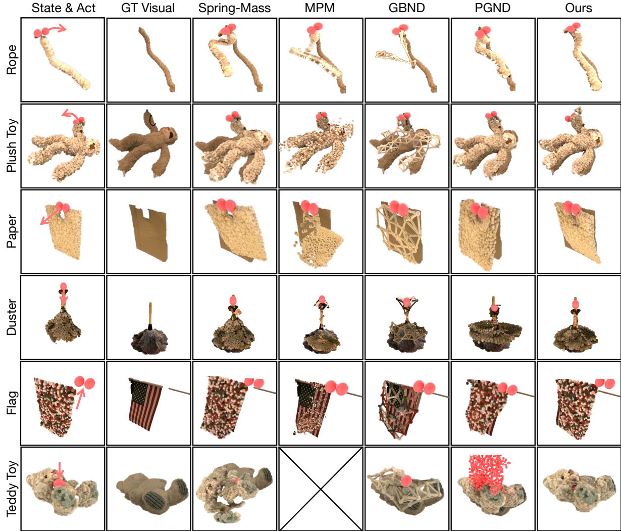
Fig. 5: Qualitative comparison on diverse objects. The first column shows the states with gripper positions (red spheres). The second column shows the GT object visualization after taking the action. PReD accurately captures deformations across all objects. For the duster, only PReD maintains stem rigidity while allowing deformation for the feathers.
